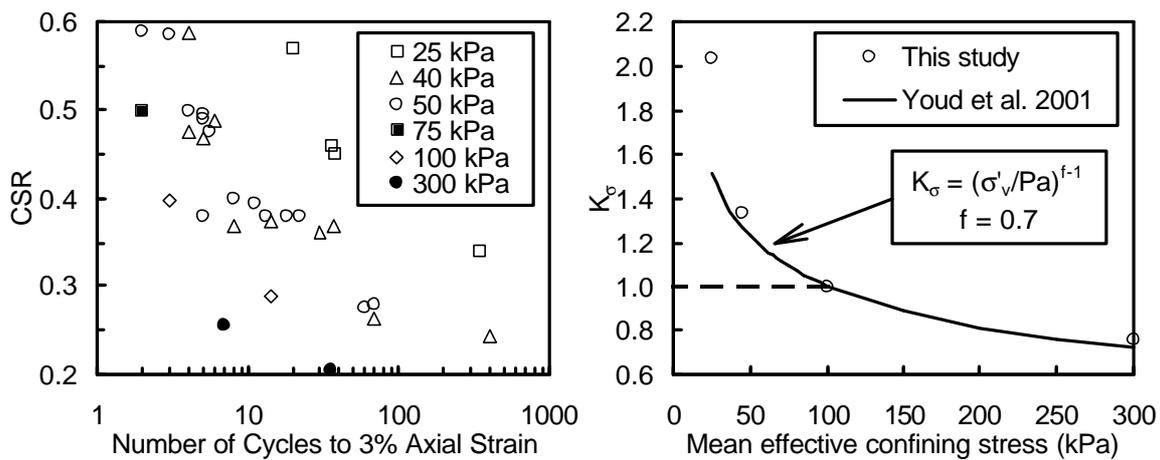
Figure 4 (a) Cyclic stress ratio (CSR) vs. number of cycles to reach 3% single amplitude axial strain for specimens of  $PI < 12$  and  $(N_1)_{60} < 10$ , tested at 25, 40, 50, 75, 100 and 300 kPa, and (b) resulting confining pressure effect.
