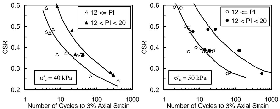
Figure 3 CSR versus number of uniform cycles to reach 3% axial strain for isotropically consolidated specimens to (a) 40 kPa and (b) 50 kPa, that have  $PI \leq 12$  (empty symbols) and  $PI > 12$ , filled in symbols. Note that soils with  $PI > 20$  did not generate significant pore pressures or axial strain.
