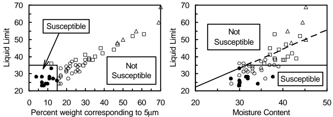
Figure 5 Graphical representation of the Chinese criteria. Specimens with  $PI \leq 12$  are shown as circles, specimens with  $12 < PI < 20$  as squares, and triangles represent soils with  $PI > 20$ . Filled in circles correspond to specimens that meet all three conditions of the Chinese criteria.
