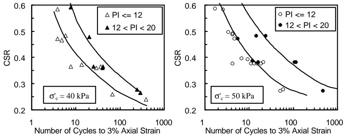
Fig. 3: CSR versus number of uniform cycles to reach 3% axial strain for isotropically consolidated specimens to (a) 40 kPa and (b) 50 kPa, that have  $PI \leq 12$  (empty symbols) and  $PI > 12$  (filled in symbols). Note that soils with  $PI > 20$  did not generate significant pore pressures or axial strain.
