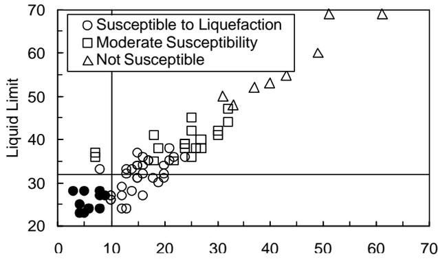
Fig. 7: Graphical representation of the Andrews and Martin criteria [6]. Filled-in circles correspond to specimens that meet the conditions of the criteria.
