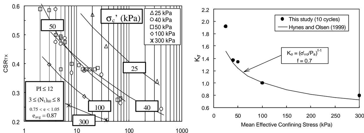
Fig. 5: (a) Number of cycles to reach 3% axial strain in extension versus applied cyclic stress ratio for specimens loaded to different hydrostatic initial effective consolidation stresses, and (b) normalized effect of confining pressure on liquefaction resistance at 10 cycles of loading for soils with low PI and penetration resistances.
