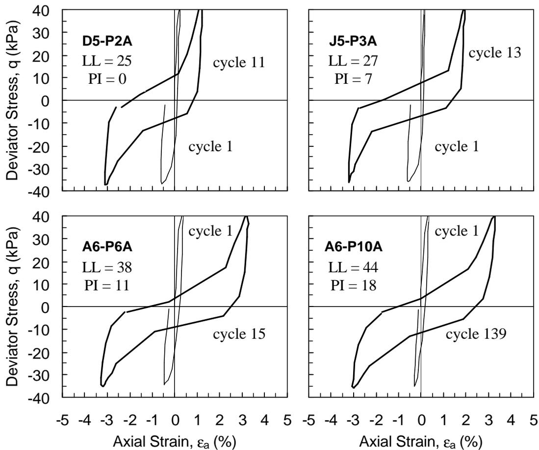
Fig. 4: Stress-strain relationship for the first cycle of loading and the cycle at which  $-3\%$  axial strain is reached for four specimens of increasing plasticity. The tests were performed on soils initially consolidated to an effective stress of 50 kPa.
