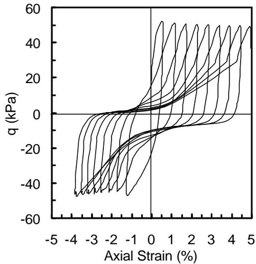
Fig. 2: Results of CTX test on non-plastic silt (LL=23) performed at  $\sigma'_c = 50$  kPa and CSR = 0.48.
