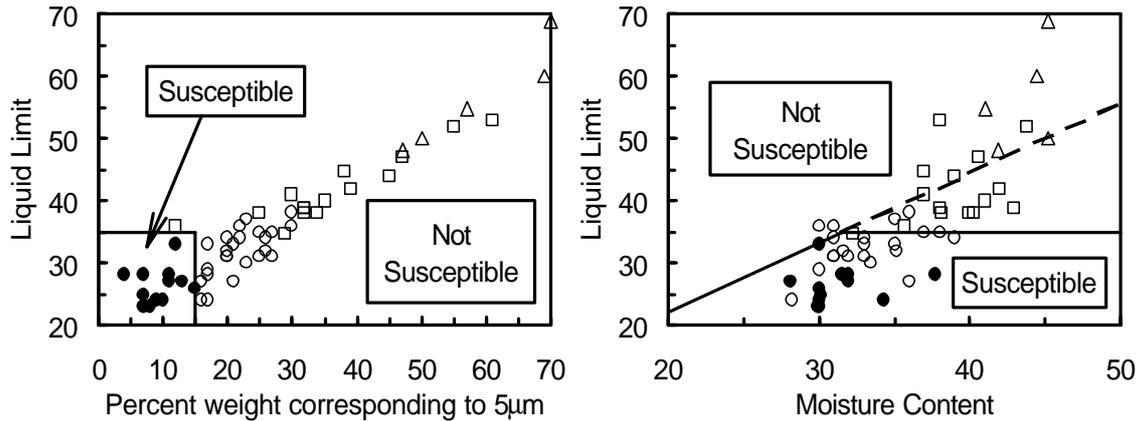
Fig. 6: Graphical representation of the Chinese criteria [2]. Test specimens susceptible to liquefaction are shown as circles; those with moderate susceptibility are shown as squares; and those not susceptible to liquefaction are shown as triangles. Only the filled symbols met all three conditions of the Chinese criteria.
