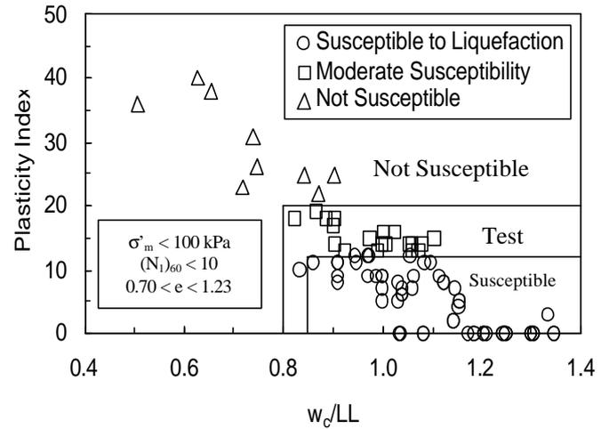
Fig. 8: Proposed criteria for the evaluation of the liquefaction susceptibility of fine-grained soils at low confining stresses.
