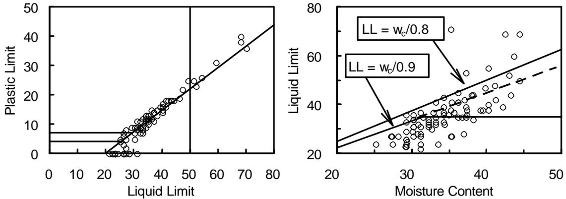
Fig. 1: (a) Location on the Casagrande plasticity chart of the soils tested in this study, (b) relationship between the LL and moisture content of the soils.
