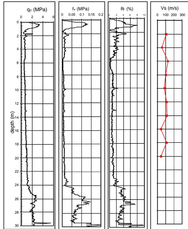
Fig. 11. A typical S-CPT record.
