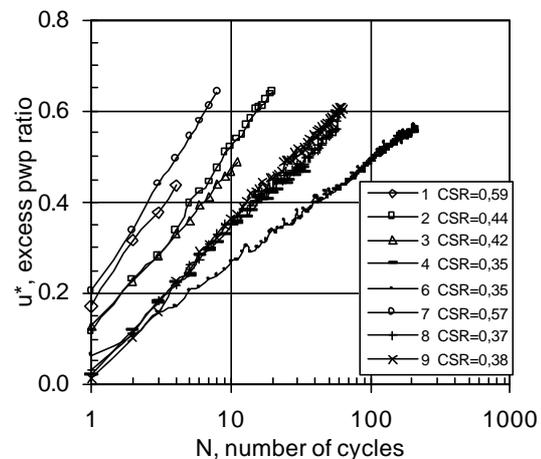
Fig. 14. Generation of residual pore water pressure
