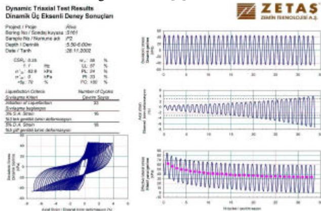
Fig. 12. Sample output of a cyclic triaxial test
