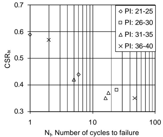
Fig. 13. Number of cycles required to reach failure condition
