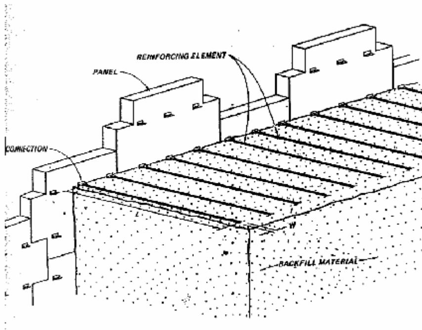
Figure 1. Schematic view of mechanically stabilized earth (MSE) wall
