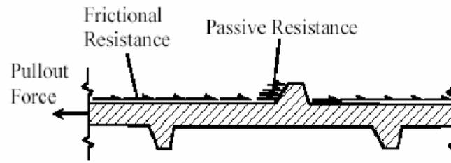
Figure 2. Longitudinal section of a strip and working principle
